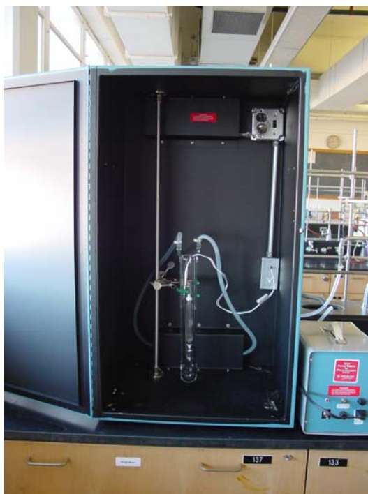
Figure 9. The mercury lamp used for the solid-state photoreaction.
